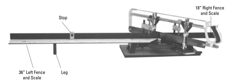
**Stop** - Allows moulding to be cut in identical lengths. **Fence and Scale** - 36" left section and 18" right section. Scale is specially designed for measuring 45° picture frame mitres.
